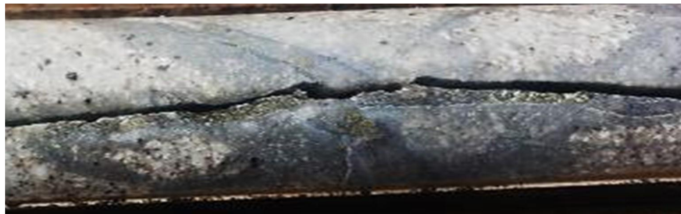
Core from BS-3 (1927.5 m) showing coarse-grained pyrite with quartz, sericite, and minor chalcopyrite (copper-iron sulfide) cutting quartz-molybdenite in quartz monzonite porphyry.
