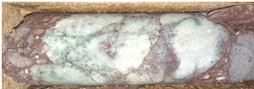
BS-4 1343m (clast in gravel) showing pervasive green sericite (phengite) replacing porphyry, overprinted by fertile red hematite likely after chalcocite derived from leached capping
